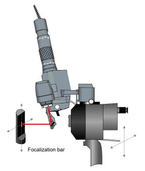
Horizontal and vertical movement of the micromanipulator
