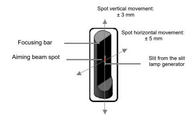
Using the micromanipulator, check that the aiming beam spot can move likewise in both horizontal and vertical directions, up the lighted slit limits.
