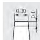
straight endgripping 0.3 mm x 0.1 mm G-36306 6 mm handle G-36308 8 mm handle
