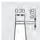
straight endgripping, extra delicate 0.2 mm x 0.05 mm G-36292 6 mm handle G-36294 8 mm handle
