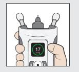
When all six measurements have been successfully taken, you hear a longer beep, the light in the probe base turns off, and you see the result on the
