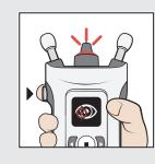
If an error occurs, the probe base flashes red. The display and sounds indicate the source of the error.
