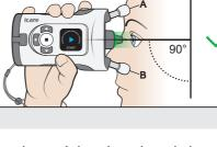
Look straight ahead and the tonometer is at a 90-degree angle to your face. The probe is about 5 mm from your eye and points perpendicularly to the center of your eye.
