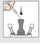
Drop the probe from the container to the probe applicator.
