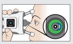
If the rings are not symmetrical, the probe does not point perpendicularly to the center of your eye. Correct the position of the tonometer.
